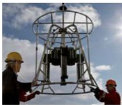
Sediment sampled: megacorer. Stations B3, B13-B18
